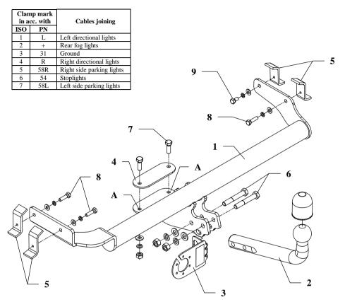
This towbar is designed to assembly in following cars: LADA SAMARA, 3/5 doors, produced since 1985 till 1998, catalogue no. N02 and is prepared to tow trailers max total weight 1100 kg and max vertical load 50 kg.
